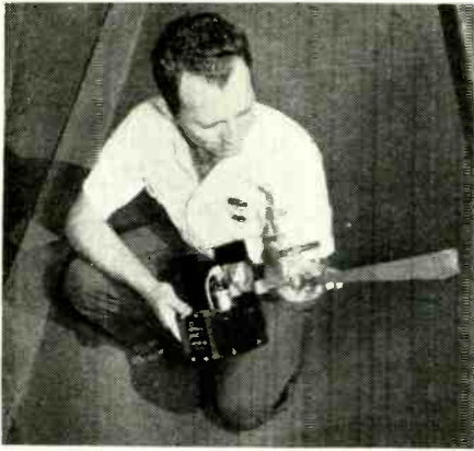
Fig. 8. Closeup of 1 cm. transmitter and horn antenna. A complete 30,000 mc. Klystron transmitter, cavity wavemeter, and high gain horn radiator makes only a light handful of microwave equipment.
