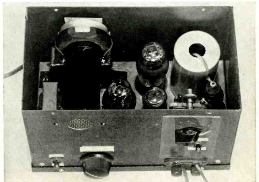
Top view of the completed condenser tester with the cover removed to show parts layout.
